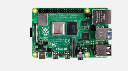
Raspberry Pi 4 Model B features a high-performance 64-bit quad-core processor, dual-display support at resolutions up to 4K via a pair of micro HDMI ports, hardware video decode at up to 4Kp60, up to 8GB of RAM, dual-band 2.4/5.0 GHz wireless LAN, Bluetooth 5.0, Gigabit Ethernet, USB 3.0, and PoE capability (via a separate PoE HAT add-on). For the end user, Raspberry Pi 4 Model B provides desktop performance comparable to entry-level x86 PC systems.
