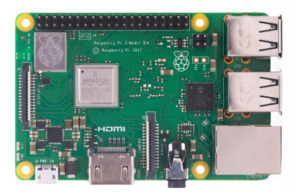
The Raspberry Pi 3 Model B+ is the latest product in the Raspberry Pi 3 range, boasting a 64-bit quad core processor running at 1.4GHz, dual-band 2.4GHz and 5GHz wireless LAN, Bluetooth 4.2/BLE, faster Ethernet, and PoE capability via a separate PoE HAT
