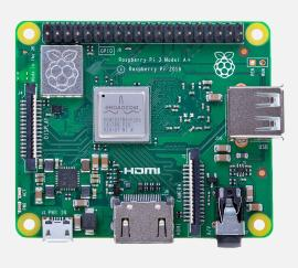
Raspberry Pi 3 Model A+, like Raspberry Pi 3 Model B+, has a 64-bit quad-core processor running at 1.4GHz, together with dual-band 2.4GHz and 5GHz wireless LAN, and Bluetooth 4.2/BLE. The dual-band wireless LAN comes with modular compliance certification.
