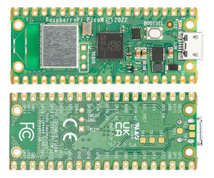
Raspberry Pi Pico W has been designed to be a low cost yet flexible development platform for RP2040, with a 2.4GHz wireless interface and the following key features:
