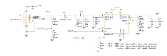
VBUS is the 5V input from the micro-USB port, which is fed through a Schottky diode to generate VSYS. The VBUS to VSYS diode (D1) adds flexibility by allowing power ORing of different supplies into VSYS.
