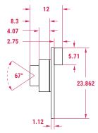
Note: all dimensions in mm tolerances are accurate to 0.2mm
