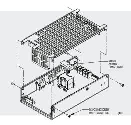
Advanced Energy's Artesyn NLP250CJ is an optional enclosure that is sold separately from the power supply. This aims to serve applications requiring physical protection from harmful environmental factors. It is recommended that effect on the power supply cooling be checked once enclosure is used.
