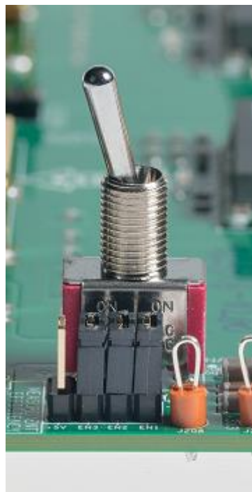
Fig. 4 – Enable jumper location and population
