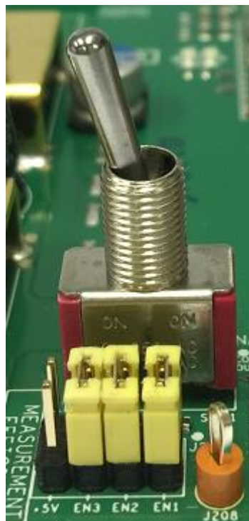
Fig. 4 – Enable jumper location and population
