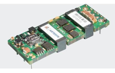
Advanced Energy's Artesyn AVO75 series of eighth-brick isolated DC-DC converters comprises six single output models offering fully regulated voltages of 1.2 V, 1.8 V, 2.5 V, 3.3 V, 5.0 V or 12.0 V. These converters can deliver up to 25 amps and up to 75 watts of output power, depending on the particular model. They have a wide 2:1 input range of 36 to 75 Vdc and are designed primarily for use with standard 48 V telecommunications equipment supplies.
