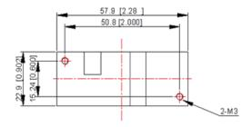
UNIT: mm[inch] BOTTOM VIEW: pin on upside TOLERANCE: X.Xmm±0.5mm[X X in.±0.02in.] XXXmm±0.25mm[X XX in.±0.01in.]
