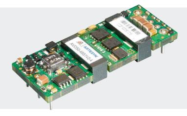
Advanced Energy's Artesyn AVO50 series of eighth-brick isolated DC-DC converters comprises seven single output models offering fully regulated voltages of 1.2 V, 1.5 V, 1.8 V, 2.5 V, 3.3 V, 5.0 V or 12.0 V. These converters can deliver up to 20 amps and up to 50 watts, depending on the particular model. They have a wide 2:1 input range of 36 to 75 Vdc and are designed primarily for use with standard 48 V telecommunications equipment supplies.
