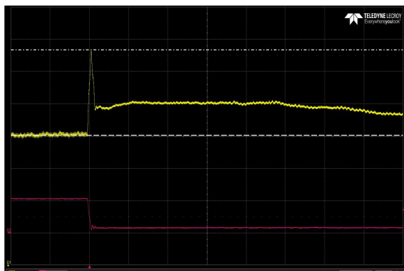
Figure 13: DS1100SLPE-3 Transient Response - V_o Deviation (high to low) 60% to 10% load change, 1A/uS slew rate, V_{IN} = 230\text{Vac} Ch 1: V_o Ch 2: I_o Output capacitance = 500uF
