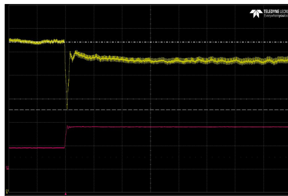
Figure 14: DS1100SLPE-3 Transient Response - V_o Deviation (low to high) 50% to 100% load change, 1A/uS slew rate, V_{IN} = 230\text{Vac} Ch 1: V_o Ch 2: I_o Output capacitance = 500uF
