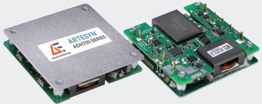
Advanced Energy's Artesyn ADH700 series half-brick isolated DC-DC converter provides a single regulated low noise output. ADH700-48S28 with 28V/25A output and ADH700-48S50 with 50V/14A output. It has a Telecom input range of 36 to 75Vdc and is designed primarily for use with standard 48 V telecommunications equipment supplies. The converter's main application area is in low power and remote radio head (RRH) telecommunications applications.
