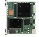
Artesyn packet processor products offer application-ready platforms for signaling and call control, network gateway and edge functions, deep packet inspection and security processing.
