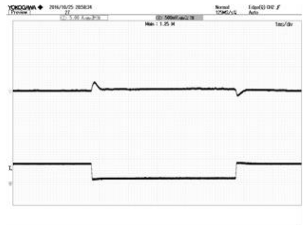
Figure 4: Dynamic response to load step 25%~75% with 0.1A/uS slew rate at 110/220Vac TOP: V_{out} , 500mV/div, BOTTOM: I_{out} , 5A/div, 1mS/div
