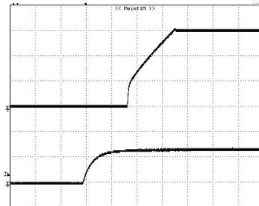
Figure 7: Turn-on transient at zero load current (5 ms/div). V_{in}=48V . Top Trace: V_{out} , 5.0V/div; Bottom Trace: ON/OFF input, 2V/div
