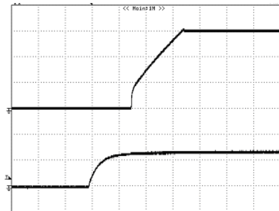
Figure 6: Turn-on transient at full rated load current (resistive load) (5 ms/div). V_{in}=48V . Top Trace: V_{out} , 5.0V/div; Bottom Trace: ON/OFF input, 2V/div
