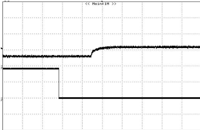
Figure 30: Turn on with Prebias 12Vin, 1.2V/0A out, V_{bias} = 0.79V_{dc} Top: 1V/div, 2ms/div, Bottom: 5V/div, 2ms/div
