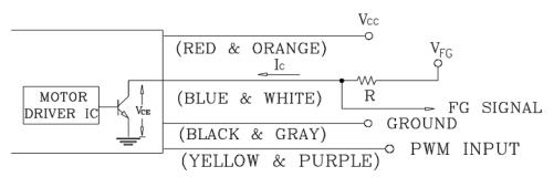
CAUTION: THE FG SIGNAL LEAD WIRE MUST BE KEPT AWAY FROM "+" LEAD WIRE & "-" LEAD WIRE.
