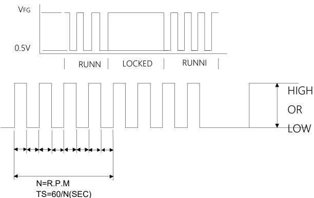
\*VFG IS ALWAYS HIGH OR LOW LEVEL AFTER BLADE LOCKED
