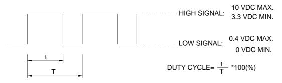
\*THE FREQUENCY FOR CONTROL SIGNAL OF THE FAN SHALL BE ABLE TO ACCEPT AT 15KHz~25KHz.
