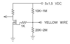
13-1. THE FAN SPEED WILL DEFAULT TO MAXIMUM WHEN THE SPEED CONTROL INPUT IS LEFT UNCONNECTED.
