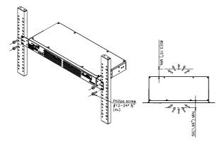
A minimum clearance is required for the rack-mount heater at both the front cool air inlet and the rear warm air exhaust, as described in the figure above, to avoid damage to the heater. Trapping warm air impacts the mechanical thermostat and cutoff thermos-fuse's judgements and causes high temperature damage to the heater. No clearance is required above or below the heater element as these surfaces are designed to remain cool during the heating operation.
