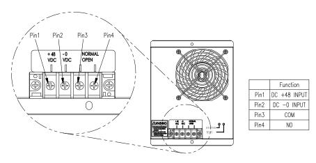
Dry contact : (Contact max. rating: <u>60VDC/50mA</u>)
