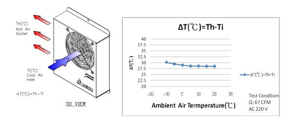
\*Note A. Minimumgapisrequiredoninletandexitpassagetoavoidtriggertheprotection of thermostat or fuse \*Note B. Do not downward the supply air to avoid short circulation
