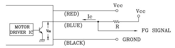
CAUTION: THE FG SINGAL LEAD WIRE MUST BE KEPT AWAY FROM"+" LEAD WIRE & "-" LEAD WIRE.
