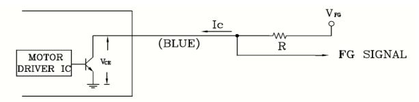
CAUTION: THE FG SIGNAL LEAD WIRE MUST BE KEPT AWAY FROM"+" LEAD WIRE & "-" LEAD WIRE.
