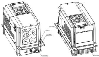
3. Install accessory 2&3 by fastening 2 of the screw 2(M6). Screw torque: 25~30kg-cm (5.21~6.94lb-in).
