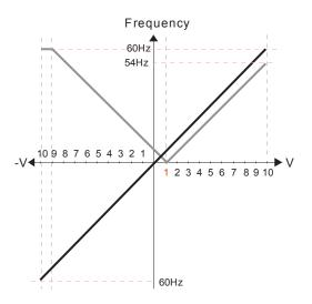
Pr.00-21=0 (Dgital keypad control and d run in FWD direction) Pr.03-05 Analog Positive Voltage Input Bias (AUI) = 10%
