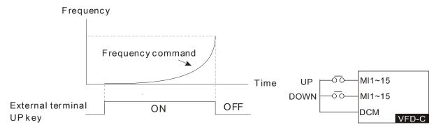
Pr.02-09 set to 1: it will increase/decrease frequency command (F) by the setting of acceleration/deceleration (Pr.01-12~01-19) and only be valid during operation.
