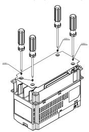
2. Install accessory 2&3 by fastening 2 of the screw 2(M6). Screw torque: 25~30kg-cm (5.21~6.94lb-in).
