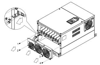
Loosen screw 1 and screw 2 (as shown in the figure below), and disconnect fan power before removing the fan. Screw torque: 24~26kg-cm (20.8~25.6in-lbf).
