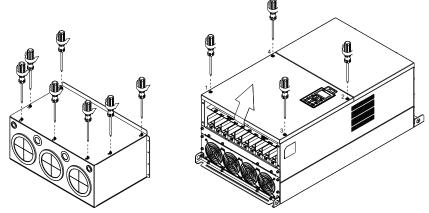
Remove the top cover and loosen the screws. Screw torque: 12~15kg-cm (10.4~13lb-in).
