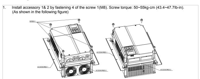
Plate installation, place 8 of the screw 2 (M6) through accessories 1&2 and the plate then fasten the screws.
