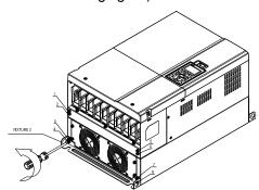
Loosen 10 screws and remove Fixture 1 (as shown in the following figure).
