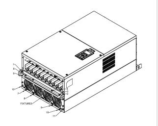
3. Loosen screw 13 ~26 and remove Fixture 1.
