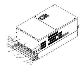
Install Fixture 1 by fasten screw 13 ~26 Screw torque: 24~26kg-cm (20.8~22.6lb-in).
