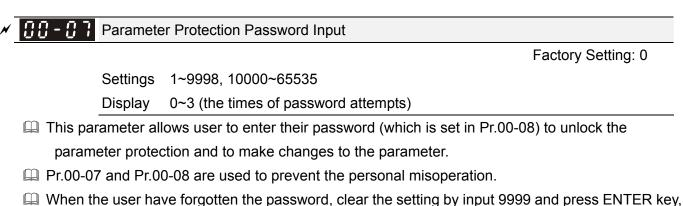
then input 9999 again and press Enter within 10 seconds. After decoding, all the settings will
