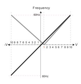
Pr.00-21=0 (Digital keypad control and run in FWD direction) Pr.03-05 Analog Positive Voltage Input Bias (AUI) = 10%
