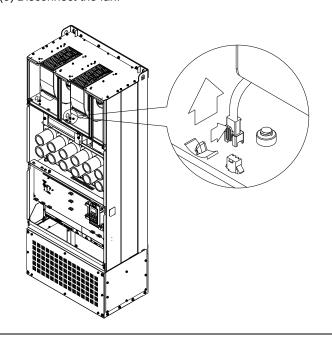
(4) Loosen the screw and remove the fan. Make sure fan power is properly disconnected before removal. Screw torque: 24~26kg-cm (20.8~22.6lb-in).
