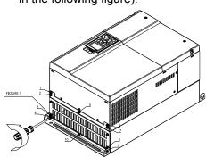
3. Fasten 4 screws (as shown in the following figure). Screw torque: 30~32kg-cm (26.0~27.8lb-in).
