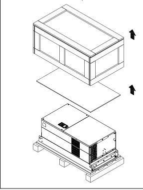
Remove the crate cover, EPEs, rubber and manual.
