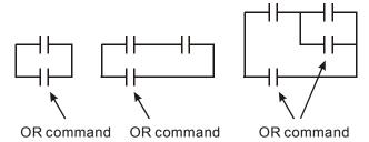
The structures of ORP and ORF are the same but the action is in rising-edge or falling-edge.
