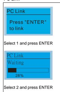
The function of PC Link is to establish a connection with computer to download the page for user defined editing. After enter to PC Link page, check if the connection of KPC-CC01 and computer is successfully establish, then press enter to go to next page and wait for communication response.
