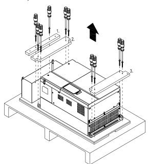
Lift the drive by hooking the lifting hole. It is now ready for installation.
