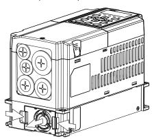
Disconnect the power terminal before removing the fan. (As shown below.)
