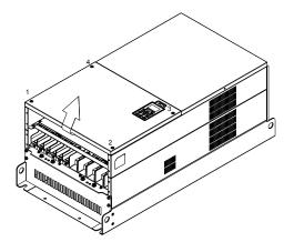
(2) For 1~8 shown in the figure: Loosen the screws Screw torque:35~40kg-cm (30.4~34.7lb-in)
