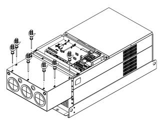
Place the cover back to the top and fasten the screws (as shown in the figure). Screw torque:  $12\sim15$ kg-cm ( $10.4\sim13$ lb-in).
