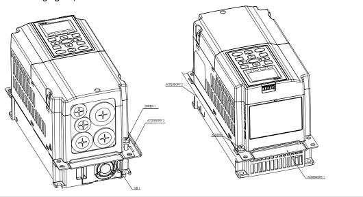
2. Install accessory 1& 2 by fastening 2 of the screw 1(M3). Screw torque: 25~30kg-cm (5.21~6.94lb-in). (As shown in following figure)
