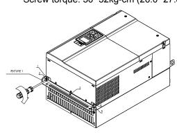
Fasten 4 screws (as shown in the following figure). Screw torque: 24~26kg-cm (20.8~22.6lb-in).
