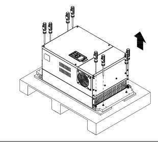
Loosen the 10 screws on the pallet and remove the wooden plate.
