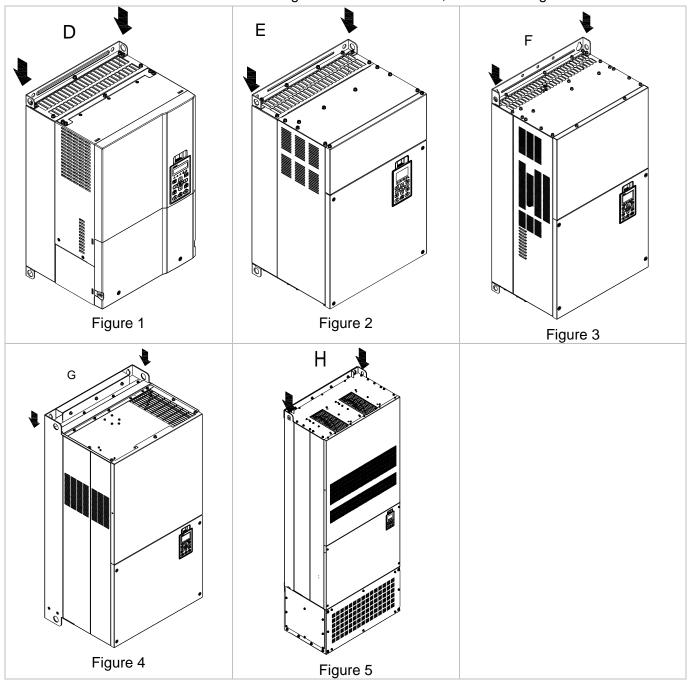
Ensure the lifting hook properly goes through the lifting hole, as shown in the following diagram. (Applicable to Frame D~G)
