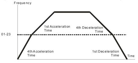
1st/4th Acceleration/Deceleration Frequency Switching
