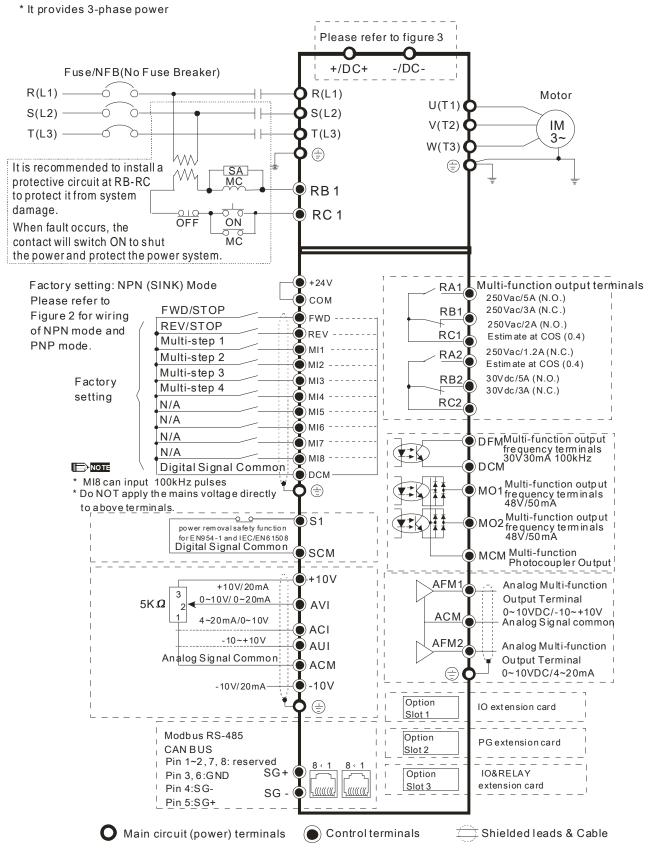
NOTE: It is recommended NOT to connect any phase advance capacitor or automatic power factor regulator (APFR) directly to the variable frequency drive. If it is necessary to connect any of them, please make sure a reactor is installed between the variable frequency drive and phase advance capacitor /APFR.
