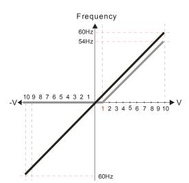
Pr.00-21=0 (Dgital keypad control and d run in FWD direction)
