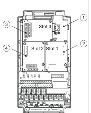
RJ45 (Socket) for digital keypad
