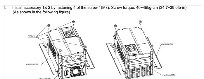
Plate installation, place 6 of the screw 2 (M6) through accessory 1&2 and the plate then fasten the screws.
