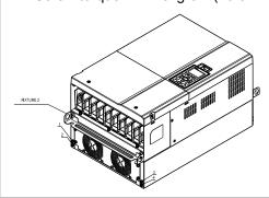
Fasten 5 screws (as shown in the following figure). Screw torque: 24~26kg-cm (20.8~22.6lb-in).
