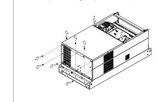
(3) Loosen screw 1,2,3 and remove the protective ring (as shown in figure below) Screw torque: 15~20kg-cm (12.2~13.9lb-in).
