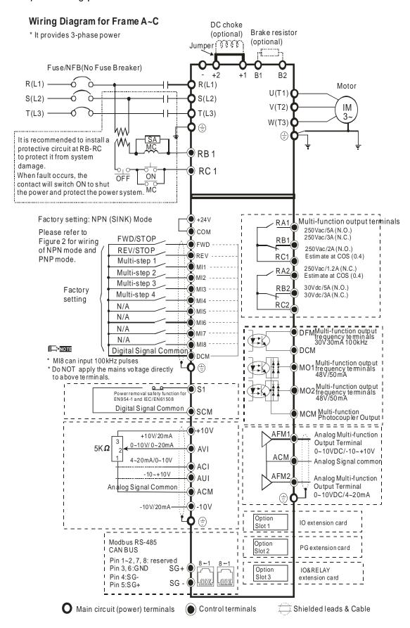
NOTE: It is recommended NOT to connect any phase advance capacitor or automatic power factor regulator (APFR) directly to the variable frequency drive. If it is necessary to connect any of them, please make sure a reactor is installed between the variable frequency drive and phase advance capacitor/APFR.
