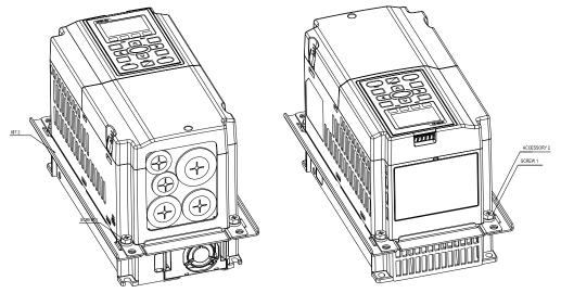
3. Plate installation, place 4 of the screw 2 (M6) through accessory 1&2 and the plate then fasten the screws. Screw torque: 25~30kg-cm (5.21~6.94lb-in). (As shown in following figure)
