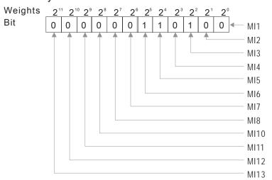
0: not used by PLC 1: used by PLC Displays = bit5x2 $^5$ +bit4x2 $^4$ +bit2x2 $^2$ = 1x2 $^5$ +1x2 $^4$ +1x2 $^2$ = 32+16+4 = 52
