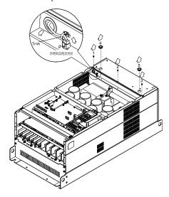
(4) Lift the fan by putting your fingure through the protective holes, as indicates in 1 and 2 on the figure.
