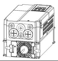
2. Disconnect the power terminal before removing the fan.
