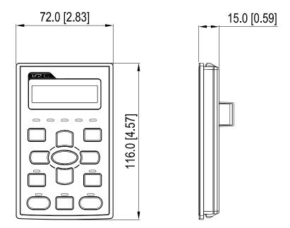
**RJ45 Extension Lead for Digital Keypad**
