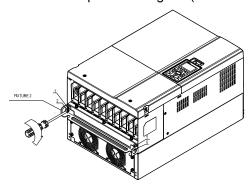
Fasten 5 screws (as shown in the following figure). Screw torque: 30~32kg-cm (26.0~27.8lb-in).
