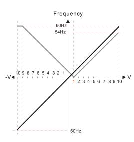
Pr.00-21=0 (Dgital keypad control and d run in FWD direction)
