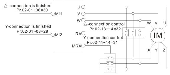
Y-  $\triangle$  connection switch: can be used for wide range motor
