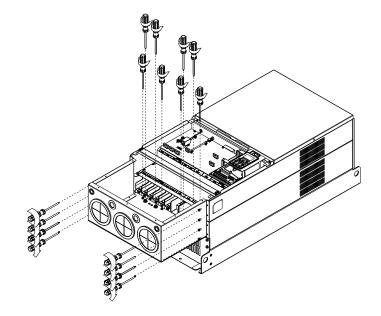
Fasten all the screws. Screw torque: 25~30kg-cm (20.8~30lb-in).
