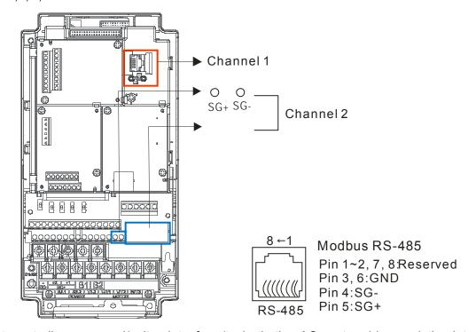
3. Host controller can read/write data from/to both the AC motor drive and the internal PLC program by setting the drive and internal PLC program to two different station numbers. For example, if user wants to set AC motor drive as station 1 and PLC as station 2, please write following setting to the host controller:
