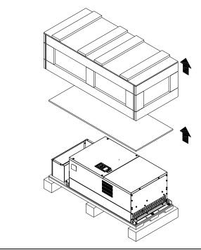
Loosen the 9 screws on the pallet and remove the wooden plate.
