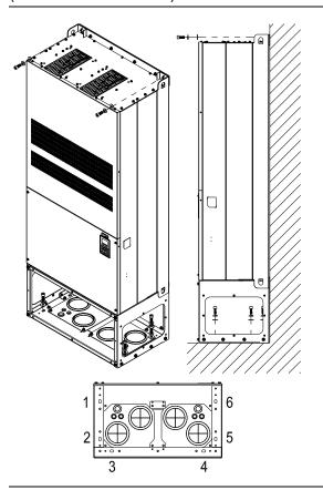
Secure the drive from the internal.
