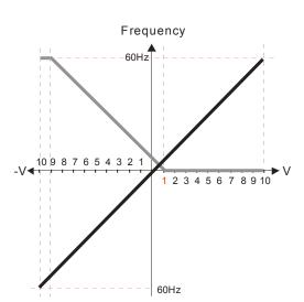
Pr.00-21=0 (Dgital keypad control and d run in FWD direction) Pr.03-05 Analog Positive Voltage Input Bias (AUI) = 10%
