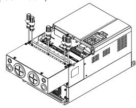
4. Fasten the 4 screws shown in the following figure. Screw torque: 10~12kg-cm (8.66~10.39lb-in).
