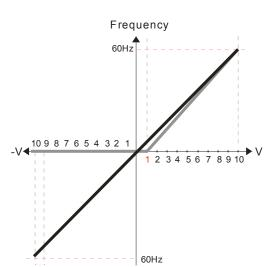
Pr.00-21=0 (Digital keypad control and run in FWD direction) Pr.03-05 Analog Positive Voltage Input Bias (AUI) = 10% Pr.03-07~03-09 (Positive/Negative Bias Mode)
