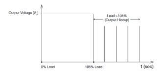
Additionally, if the lo is <250% but >110% for a prolong period of time (depending on the load), the Over Temperature Protection (OTP) will be activated due to high temperature on critical components. The power supply will then go into hiccup mode until the fault is removed; and, the input voltage is removed, then reapplied.
