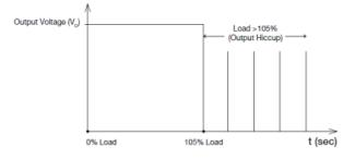
Additionally, if the I<sub>0</sub> is <250% but >110% for a prolong period of time (depending on the load), the Over Temperature Protection (OTP) will be activated due to high temperature on critical components. The power supply will then go into hiccup mode until the fault is removed; and, the input voltage is removed, then reapplied.
