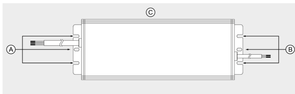
Fig. 3 Mounting Hole Locations
