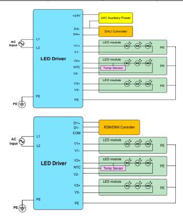
**Note:** All the output channels are independent, any series or parallel connections are not allowed, the user should strictly follow the connection schematic.
