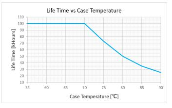
Note: Test at input voltage 220Vac & 400Vac, at full Load with each channel 2.0A/350V.
