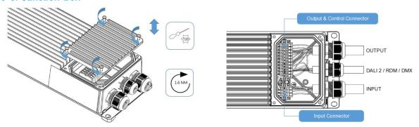
Note: The cap and fastening 4 screws all have the function of anti-falling off.
