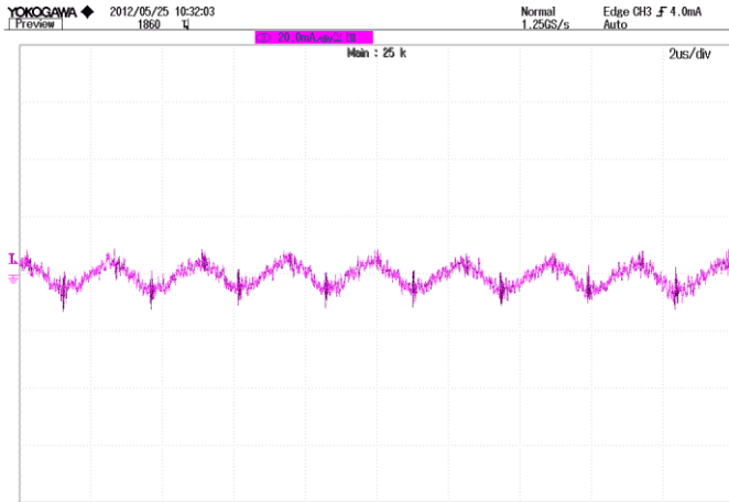
Figure 12: Input reflected ripple current, i_s , through a 12\mu\text{H} source inductor at nominal input voltage and max load current (20 mA/div, 2us/div).
