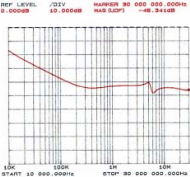
Figure 2: Typical differential-mode insertion loss in a 50Ω circuit
