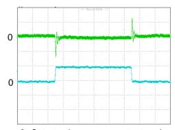
Figure 9: Output voltage response to step-change in load current (75%-50%-75% of lo, max; di/dt = 1.0A/µs). Load cap: 10µF tantalum capacitor and 1µF ceramic capacitor. Top Trace: Vout (100mV/div, 200us/div), Bottom Trace: lout (10A/div). Scope measurement should be made using a BNC cable (length shorter than 20 inches). Position the load between 51 mm to 76 mm (2 inches to 3 inches) from the module
