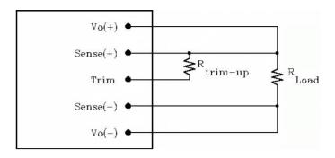
Figure 18: Circuit configuration for trim-up (increase output voltage)
