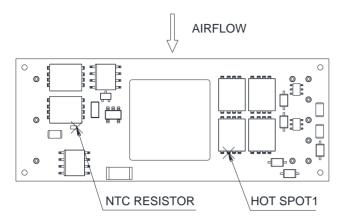
**Figure 20:** \* Hot spot 1& NTC resistor temperature measured points. The allowed maximum hot spot 1 temperature is defined at 117  $^{\circ}$ C
