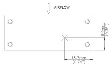
**Figure 22:** \* Hot spot 2 temperature measured point. The allowed maximum hot spot 2 temperature is defined at 105  $\mathcal C$
