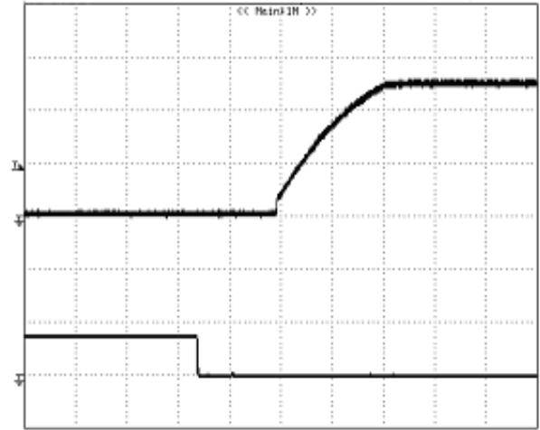
Figure 5: Turn-on transient at full rated load current (constant current load) (5 ms/div). V_{in}=48V . Top Trace: V_{out} , 2V/div; Bottom Trace: ON/OFF input, 5V/div.
