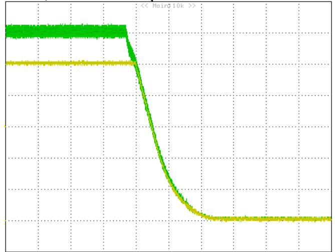
Figure 24: Tracking function, V_{tracking}=6V , V_{out}= 5.0V , full load Yellow : V_{OUT} , (1V/div), Green: Tracking, (1V/div), 10mS/div
