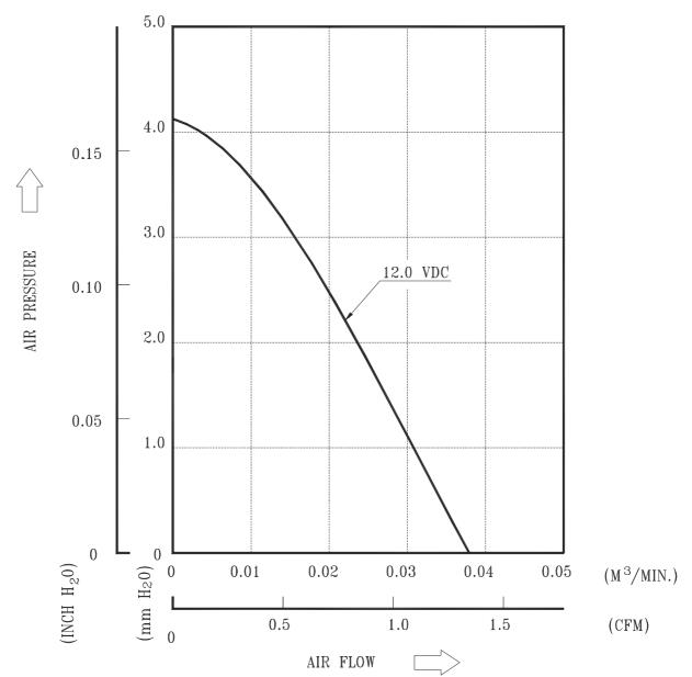
\*TEST CONDITION: INPUT VOLTAGE-----OPERATION VOLTAGE
