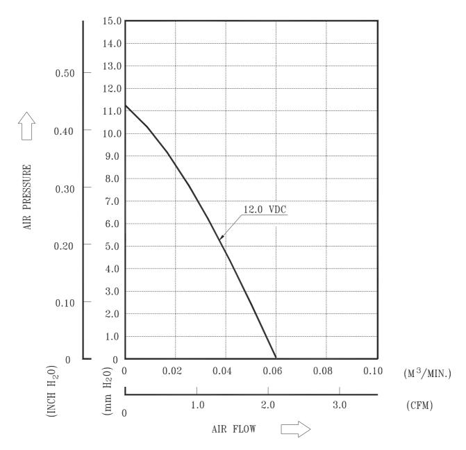
\*TEST CONDITION: INPUT VOLTAGE-----OPERATION VOLTAGE
