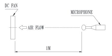
NOISE IS MEASURED AT RATED VOLTAGE IN FREE AIR IN ANECHOIC CHAMBER WITH B & K SOUND LEVEL METER WITH MICROPHONE AT A DISTANCE OF ONE METER FROM THE FAN INTAKE.
