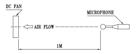
NOISE IS MEASURED AT RATED VOLTAGE IN FREE AIR IN ANECHOIC CHAMBER WITH B & K SOUND LEVEL METER WITH MICROPHONE AT A DISTANCE OF ONE METER FROM THE FAN INTAKE. PART NO:
