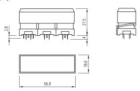
4 keylock switch 2 positions, keylock switch 3 positions page 535, 536
