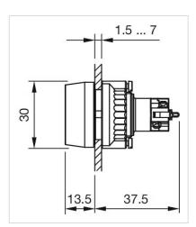
Illuminated pushbutton, Momentary, 250 V AC @ 3 A, 24 V AC/DC, 1 NC / 1 NO, Soldering terminal, round, Blue, Blue
