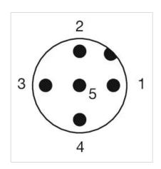
1 = NC 2 = LED+ 3 = Common 4 = LED-5 = NO A-Coded
