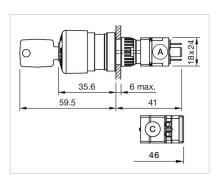
A = Plug-in terminal 2.8 mm x 0.5 mm C = Screw terminal
