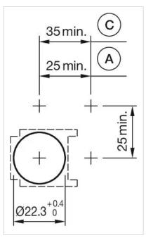
$\label{eq:A} A = Solder/Plug-in terminal 2.8 mm x 0.5 mm \\ C = Screw terminal$
