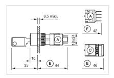
A = Plug-in terminal 2.8 mm x 0.5 mm C = Screw terminal E = Slow-make switching element F = Snap-action switching element
