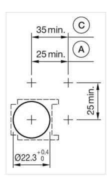
A = Solder/Plug-in terminal 2.8 mm  $\times$  0.5 mm
