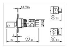
$\label{eq:Absolute} \begin{array}{l} A = \mbox{Plug-in terminal } 2.8 \mbox{ mm x } 0.5 \mbox{ mm} \\ C = \mbox{Screw terminal} \end{array}$
