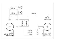
A = Solder/Plug-in terminal 2.8 mm x 0.5 mm C = Screw terminal
